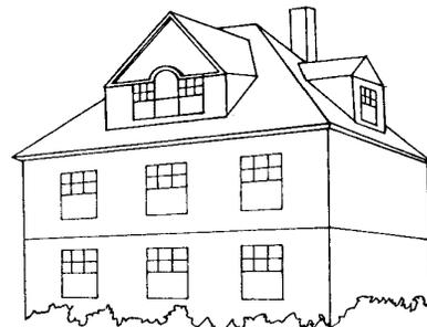
*Figure 15: Gable dormer windows should not extend into the pediment wall surface above unless deemed appropriate for the building style, such as this three-part Palladian window in a Colonial Revival house. Dormer windows should be balanced in proportion with the windows in the main wall beneath them.*
