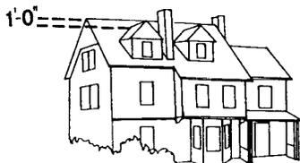
**Figure 12:** Gable dormers added in combinations, such as pairs, should not exceed 15 ft. in total length. The preferred setback from the roof ridge should be at least 1 foot.
