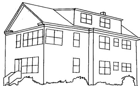
**Figure 8:** The preferred location for a larger single dormer on a gable-front building is offset toward the rear.
