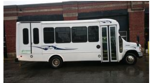
Utilizing a Massachusetts Division of Energy Resources Green Communities Grant, Public Works was able to convert two maintenance vans, a shuttle bus (above), and a trash truck to hybrid drive systems to reduce tailpipe emissions and the use of fossil fuels.
