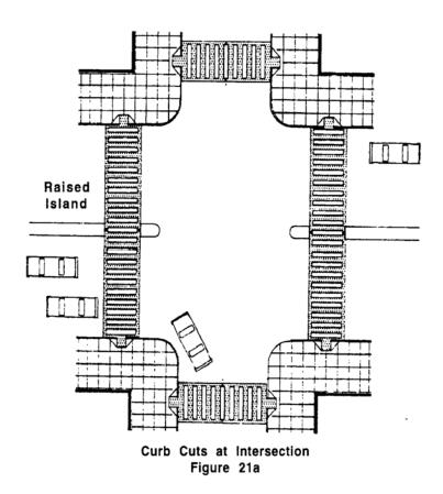
Exception: Where pedestrian right-of-way established width will not accommodate a perpendicular *curb cut* and landing, a parallel public *sidewalk curb cut* with a *level* landing at its bottom shall be provided instead of a perpendicular *curb cut*.
