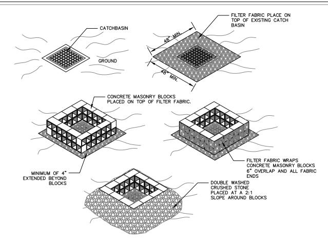
THIS METHOD OF INLET PROTECTION IS APPLICABLE WHERE HEAVY FLOWS ARE ANTICIPATED AND OVERFLOW CAPACITY IS NECESSARY TO PREVENT EXCESSIVE PONDING
