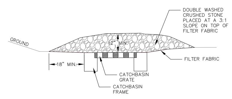
THIS METHOD OF INLET PROTECTION IS APPLICABLE WHERE HEAVY FLOWS ARE ANTICIPATED BUT NOT WHERE PONDING AROUND THE STRUCTURE MIGHT CAUSE EXCESSIVE DAMAGE TO ADJACENT STRUCTURES AND UNPROTECTED AREAS.
