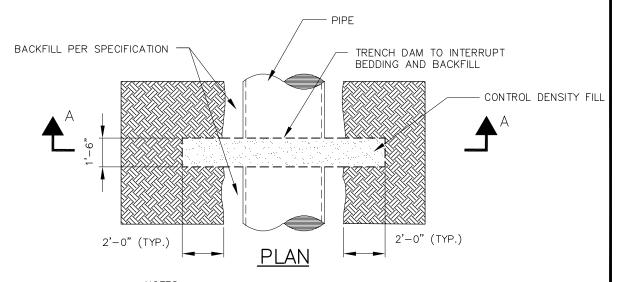
NOTES: 1. NOTCH TRENCH DAM A MINIMUM OF 2'-0" BEYOND UNDISTURBED MATERIAL ON SIDES AND BOTTOM OF
