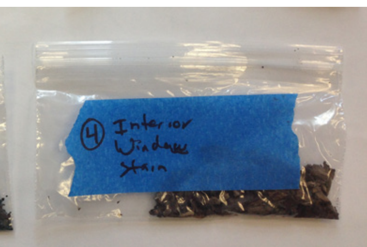
Existing paint samples for lead testing.
