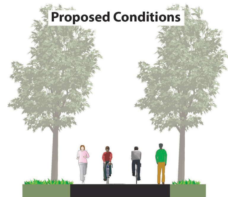
Paths 11' - 14.5' operate with two travel lanes and one shared central pass lane
