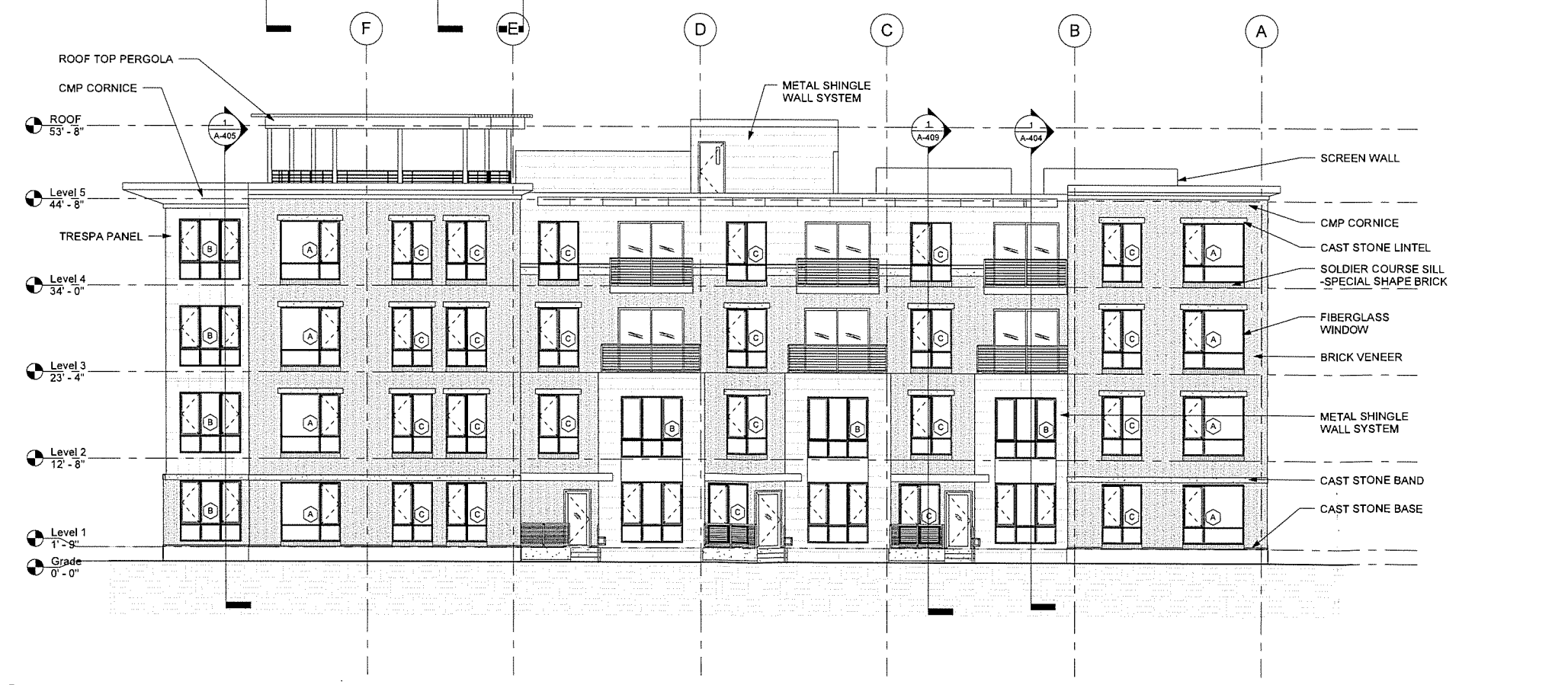
2 NORTH ELEVATION (BENT STREET) 1/8" = 1'-0"
