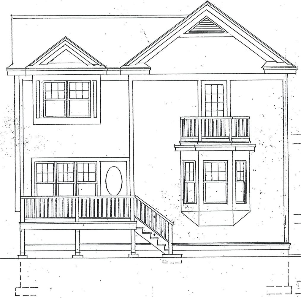
REAR ELEVATION SCALE 1/4" = 1'-0"
