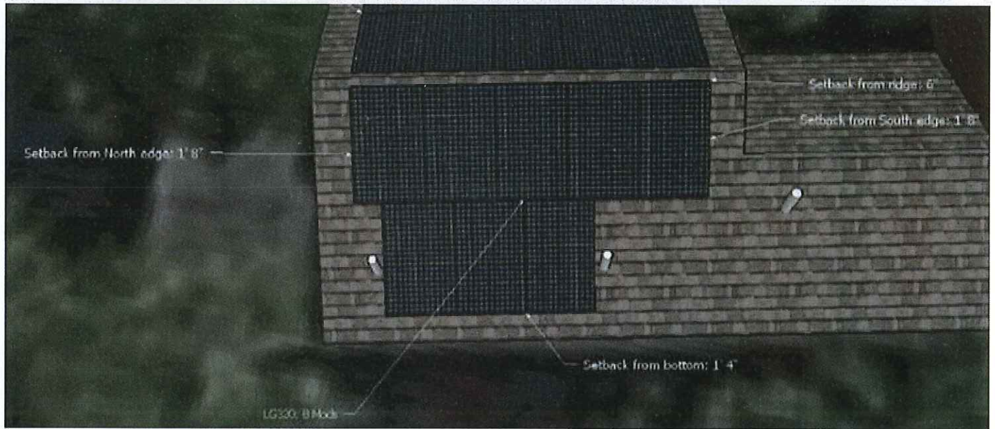
SW Layout: Panels are 4" above roof deck, no rails visible
