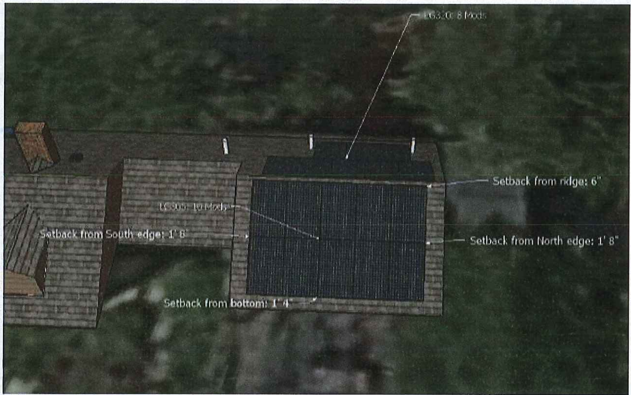
SW Layout: Panels are 4" above roof deck, no rails visible
