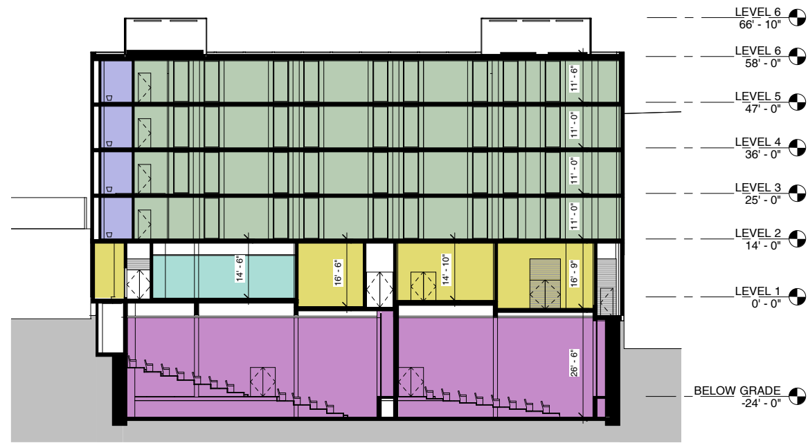
Building Section B Scale 1/32" = 1'-0"
