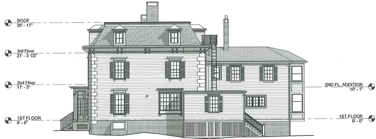
W West Elevation - Existing 1/16" = 1'-0"
