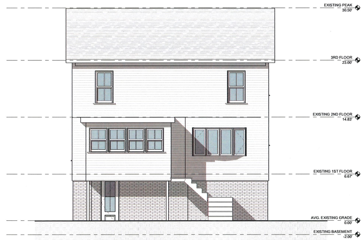
① FRONT ELEVATION - EXISTING 1/4" = 1'-0"
