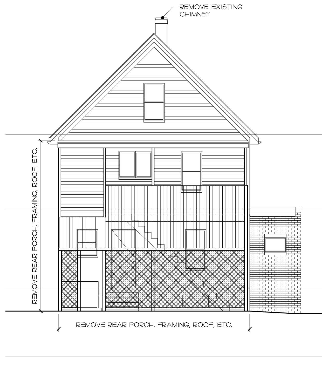
6 EXISTING/DEMO NORTH/REAR ELEVATION Scale: 3/16" = 1'-0"
