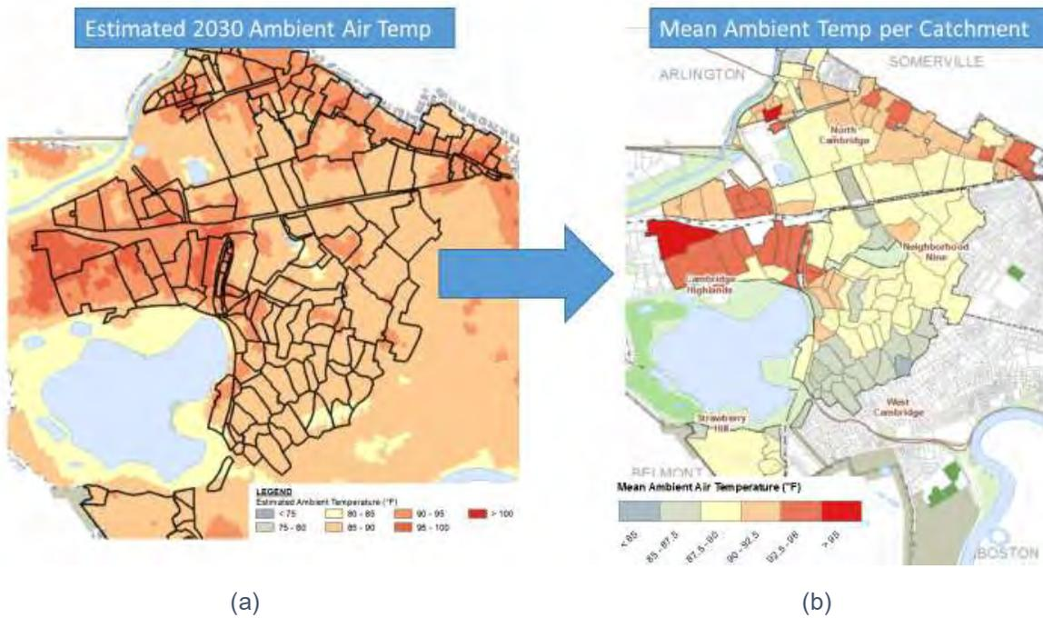
Figure 10. 2030 ambient air temperature (a) as determined in the CCVA study, and (b) summarized at the subcatchment scale under existing conditions with no green infrastructure
