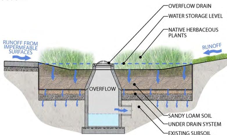
**Figure 2: Bioretention Basin Typical Section**
