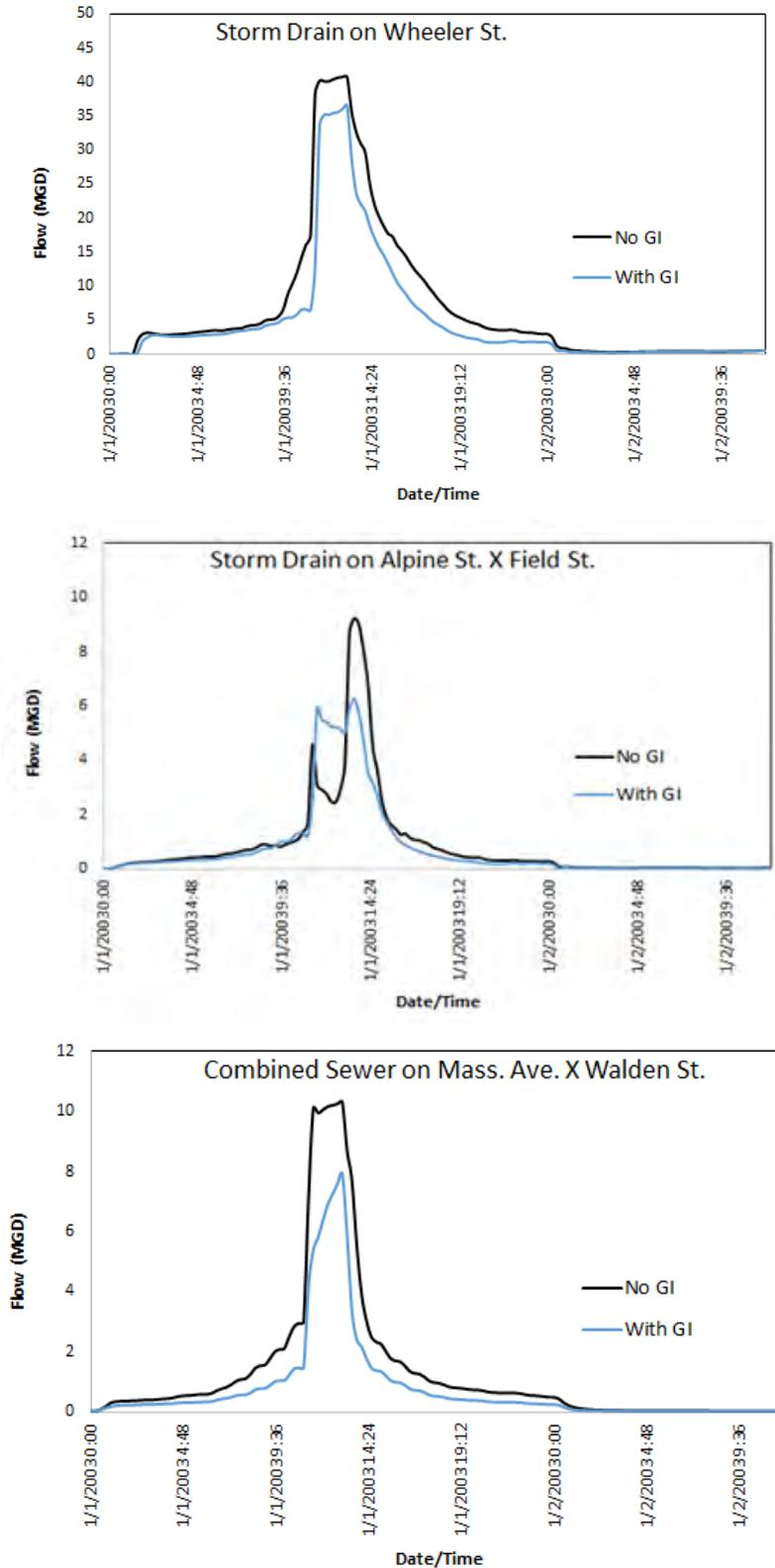
**Figure 3.** Flow hydrographs for the 10-year, 24-hour under 2070 horizon with and without GI implementation in Alewife.
