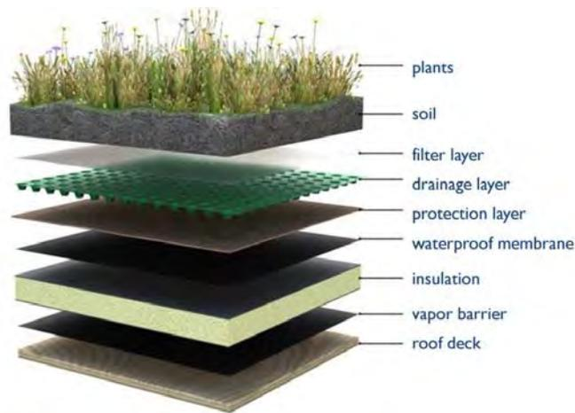
**Figure 9: Typical Extensive Green Roof Section**
