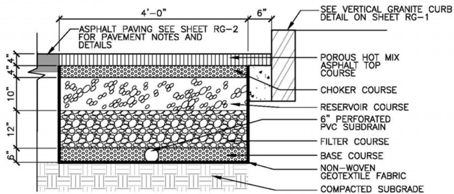
**HOT MIX ASPHALT POROUS PAVING (36" DEPTH, 4' WIDTH)**
