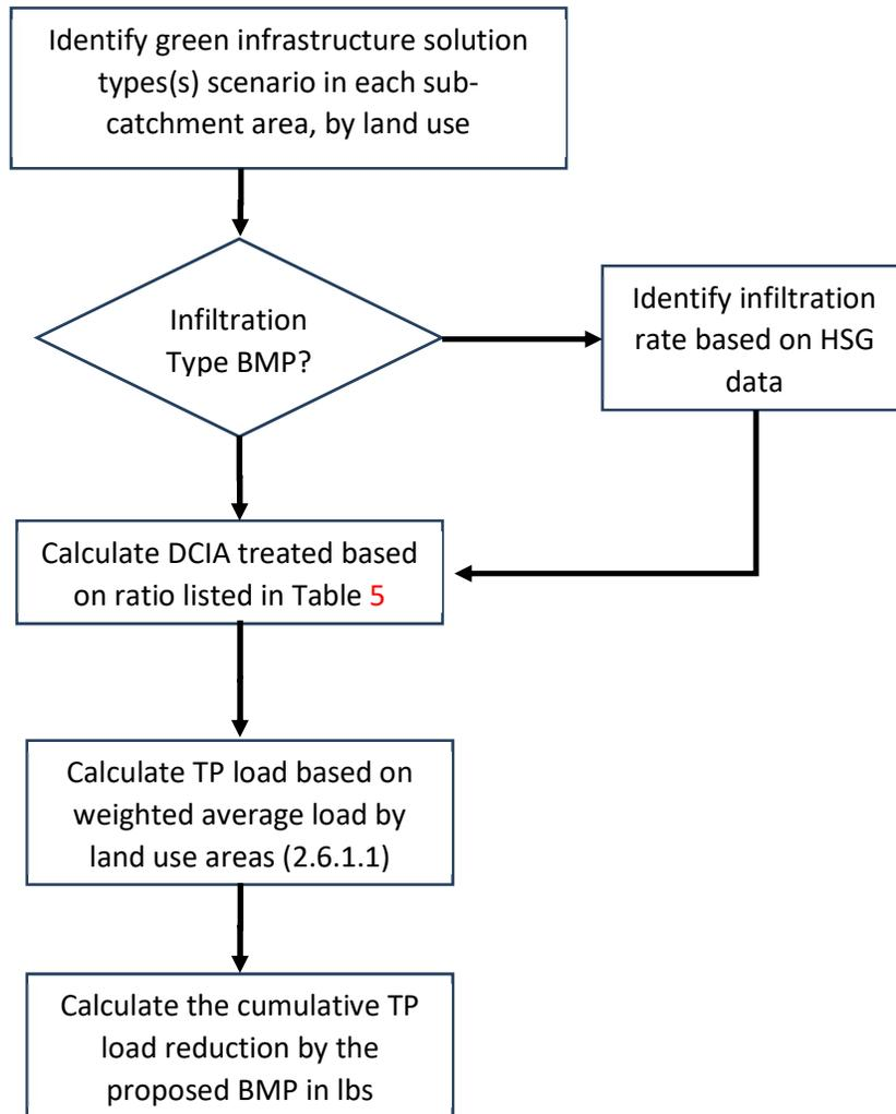
**Figure 5: Flow Chart of Method to Determine Total Phosphorus Load Reduction Based on known BMP Implementation Level**
