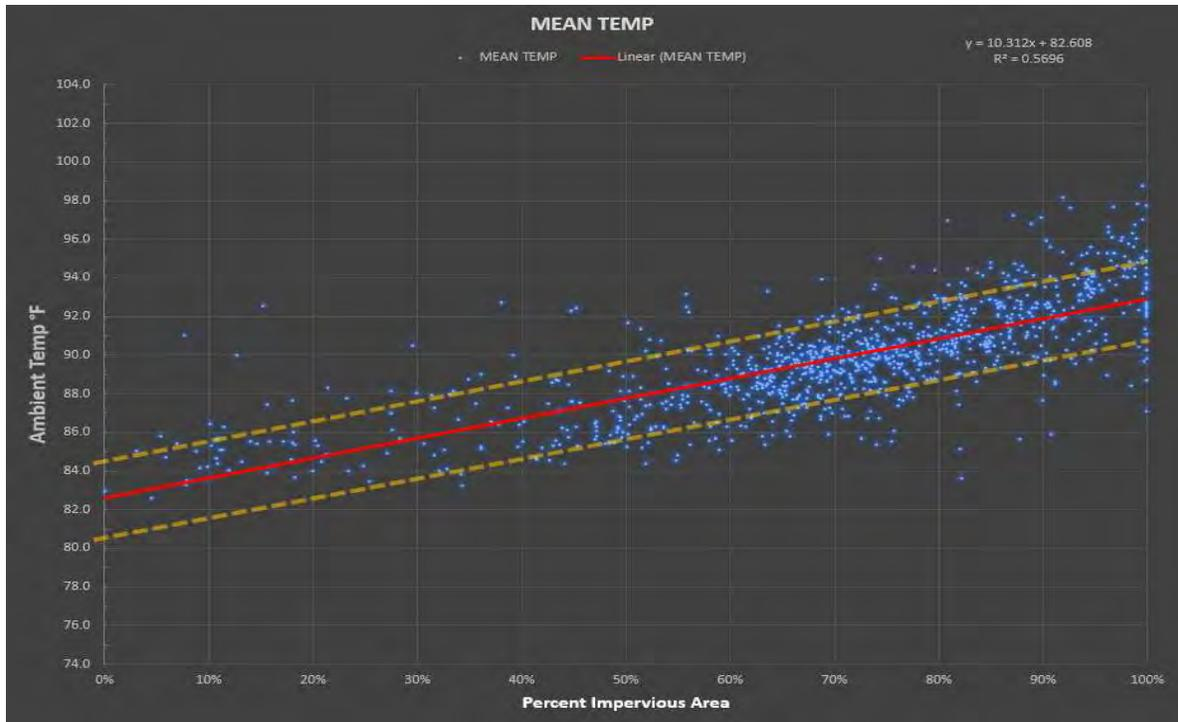
Figure 11: Relationship between ambient air temperature and percent imperviousness under existing conditions
