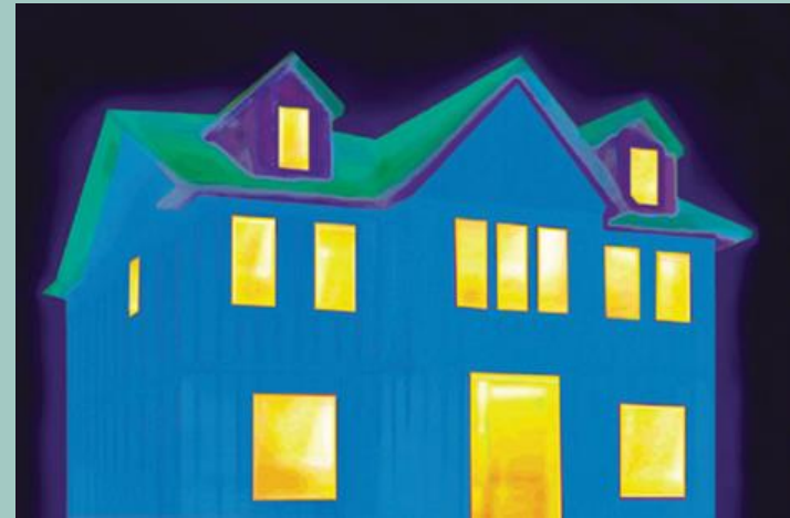
Reduced thermal bridging with continuous exterior insulation
