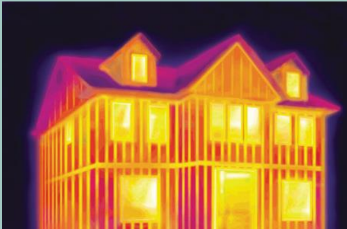
Thermal bridging in a wood-framed house
