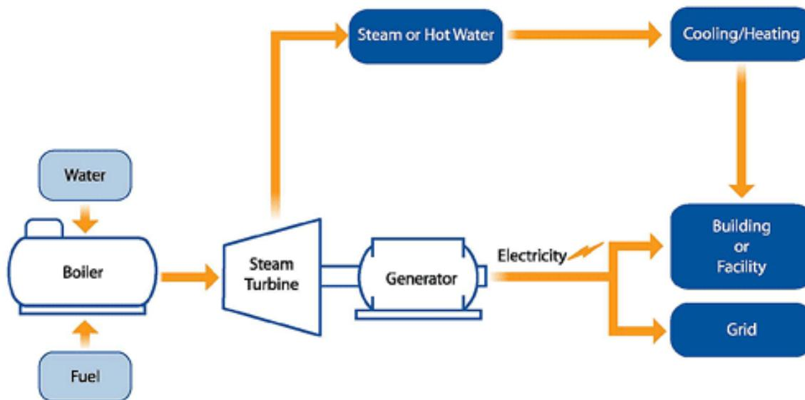
**Figure 4: Typical Steam Generation System<sup>27</sup>**
