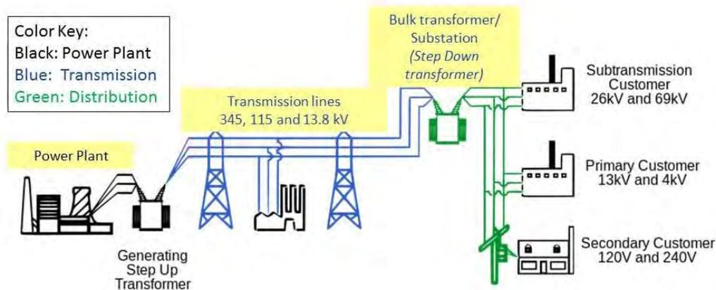
**Figure 1: Diagram of Electricity Generation, Transmission, and Distribution<sup>10</sup>**
