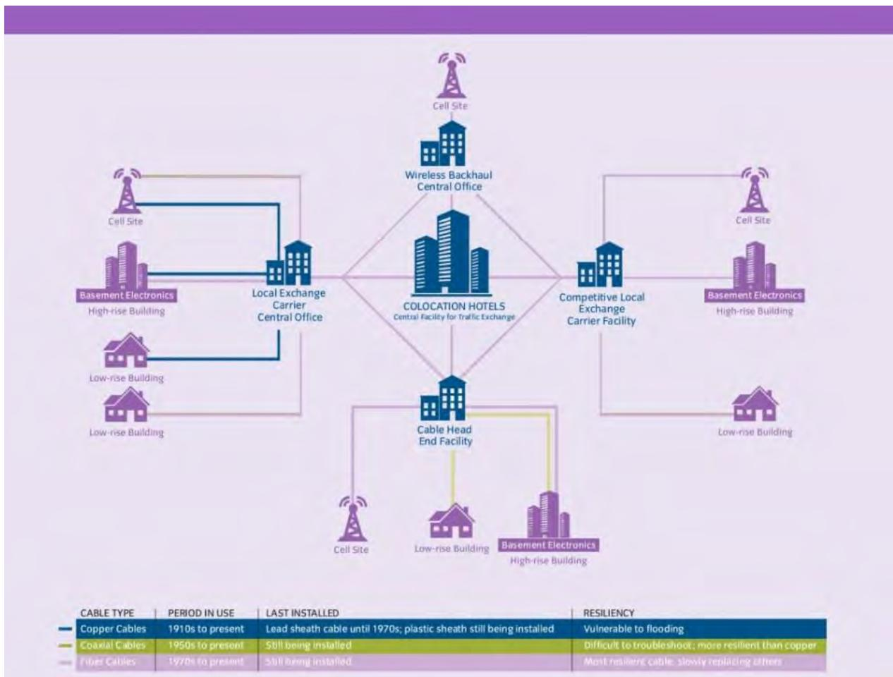
Figure 1: Diagram of Telecommunications Components<sup>98</sup>.
