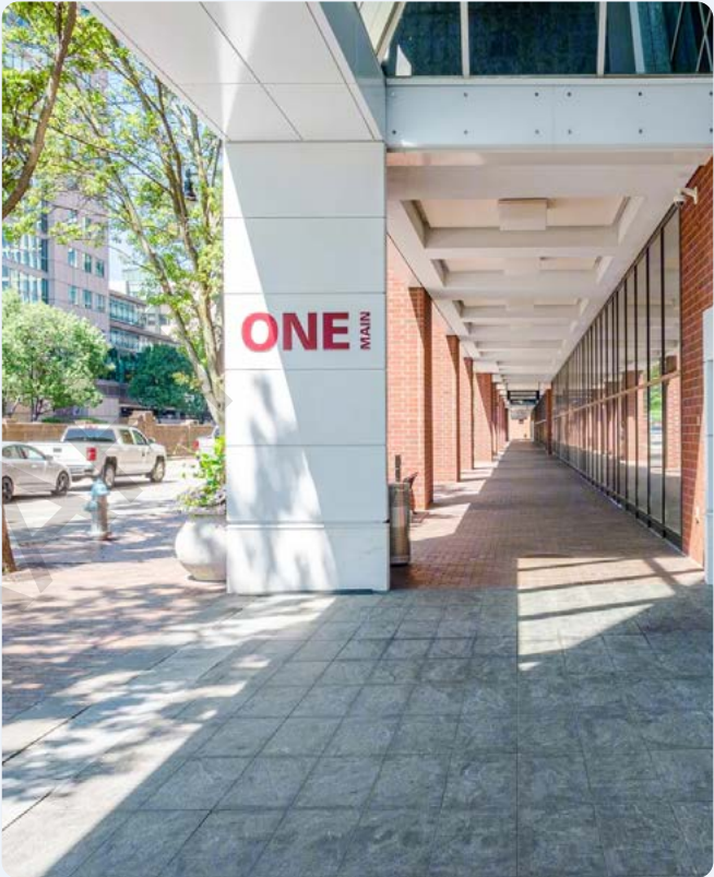
FIG. 25 Colonnades along the streets can improve pedestrian wind conditions.
