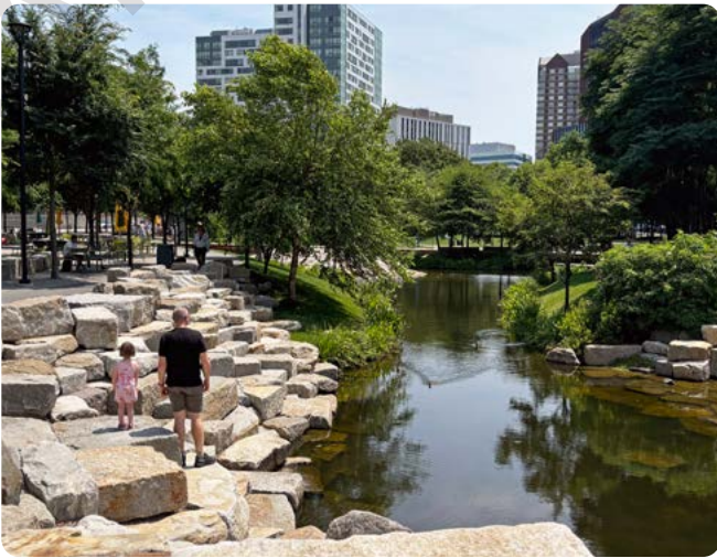
FIG. 100 The Common at Cambridge Crossing features retention ponds that help improve the water quality from stormwater runoff.
