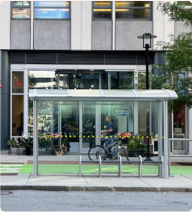
FIG. 220 Visually transparent bus shelter in Kendall Square enhances safety and visibility for all users. The stop also features a floating design that separates bus passengers from the bicycle lane, improving both comfort and circulation.
