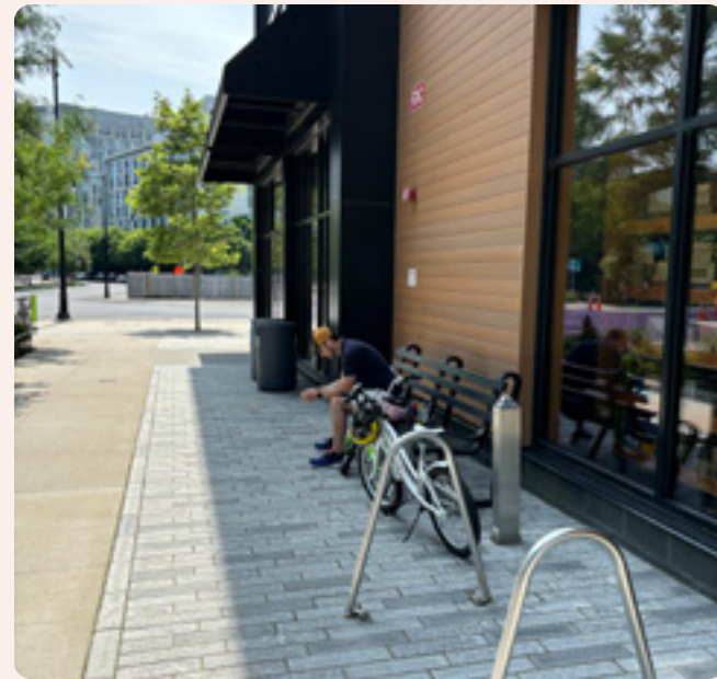
FIG. 204 Pavers demarcate the privately owned Frontage Zone, while complementing other sidewalk paving materials.
