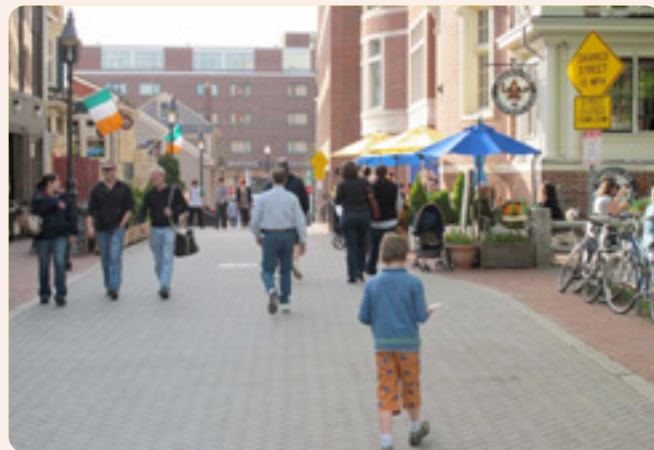
FIG. 177 Winthrop St, a commercial shared street, uses flush gray concrete and red brick pavers to reinforce its pedestrian-priority.
