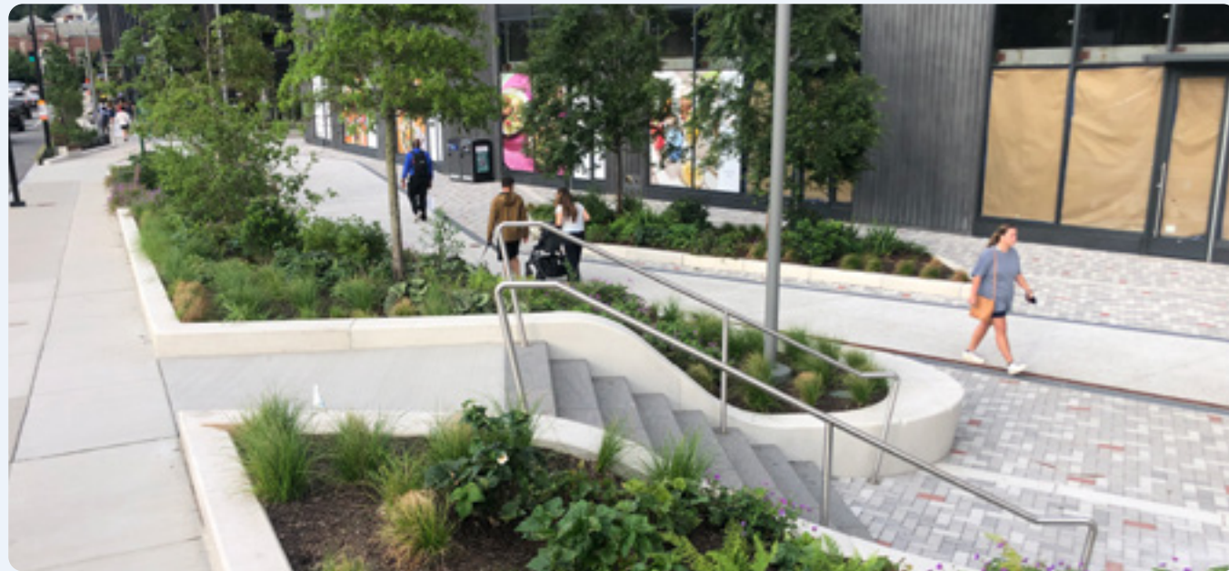
FIG. 17 Permeable planted areas and light colored paving are used in combination with trees at the Union Square development in Somerville.
