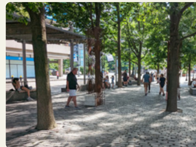
FIG. 111 At Central Wharf Plaza in Boston, a clear walking path and a furnished edge work together to create a safe, comfortable separation between people walking and vehicles.
