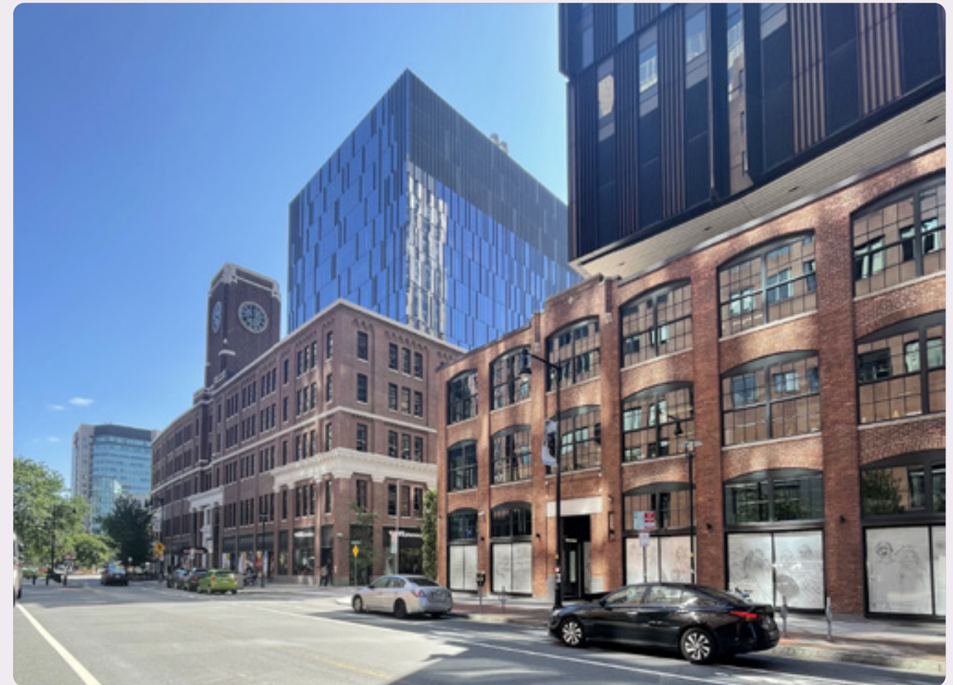
FIG. 38 Towers of tall buildings in Kendall Square step back from the street to mediate between the scale of people walking and the building's bulk.
