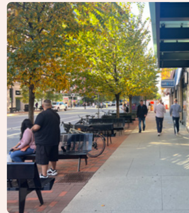
FIG. 211 Benches, bicycle racks, street trees, and brick paving define the Planting/Furnishings Zone in Kendall Square.
