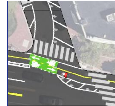
"Squaring Up" Large Angles with Flex Posts
