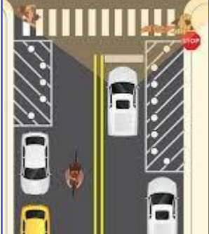
Removing Parking for Daylighting
