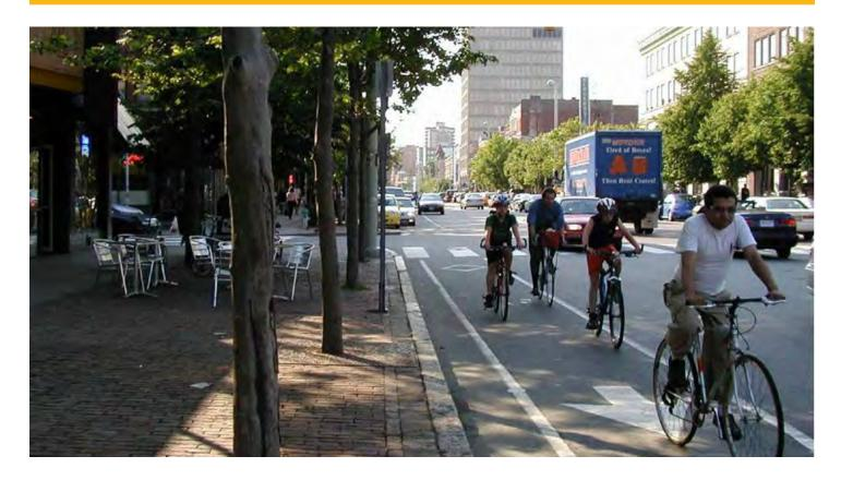
Bike lanes designate an exclusive space for bicyclists through the use of pavement markings and signage. The bike lane is located adjacent to motor vehicle travel lanes and flows in the same direction as motor vehicle traffic. Bike lanes are typically on the right side of the street. Benefits include providing obvious space on the road for cyclists and sending a message to other road users to expect cyclists.
