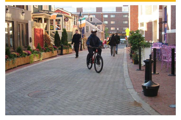
A shared street in this meaning is one where there is no curbed delineation between the roadway and the sidewalk and all users share the space. Vehicle volumes are either low or discouraged. The concept is also known as a "woonerf" (a Dutch term loosely translated into "living street").
