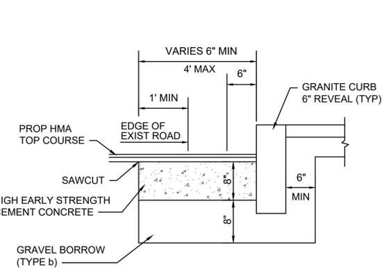
**GRANITE CURB IN FULL DEPTH PAVEMENT LESS THAN 4' WIDE**
