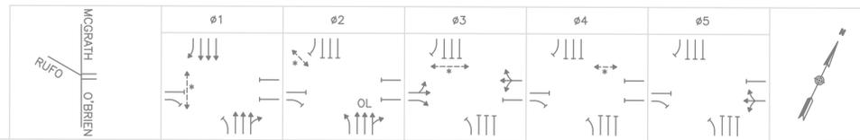
SEQUENCE AND TIMING FOR FULLY ACTUATED CONTROL (COORDINATED)
