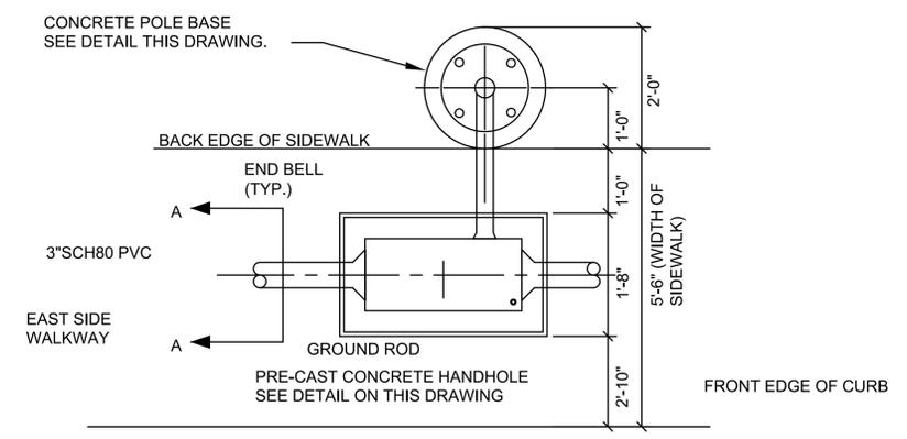
TYPICAL HANDHOLE AND POLE ARRANGEMENT NOT TO SCALE
