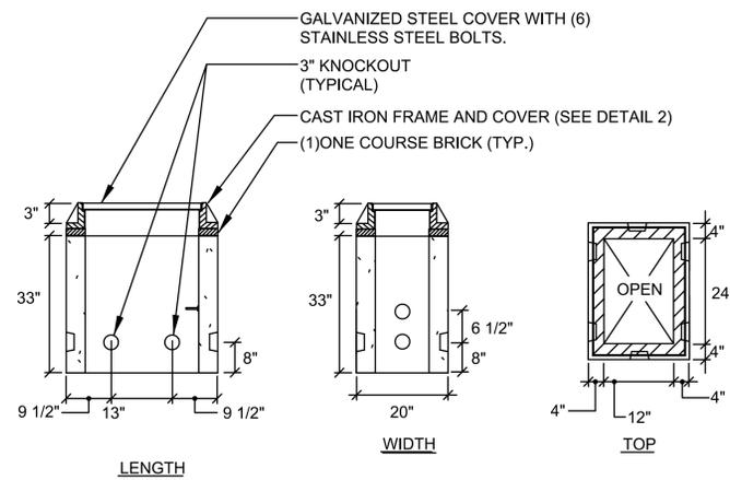
TYPICAL PRE-CAST CONCRETE HANDHOLE NOT TO SCALE
