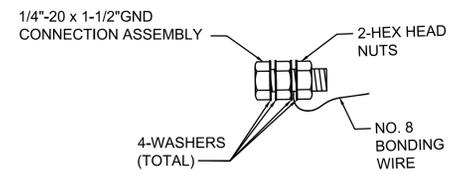
GALVANIZED STEEL BONDING TAB NOT TO SCALE
