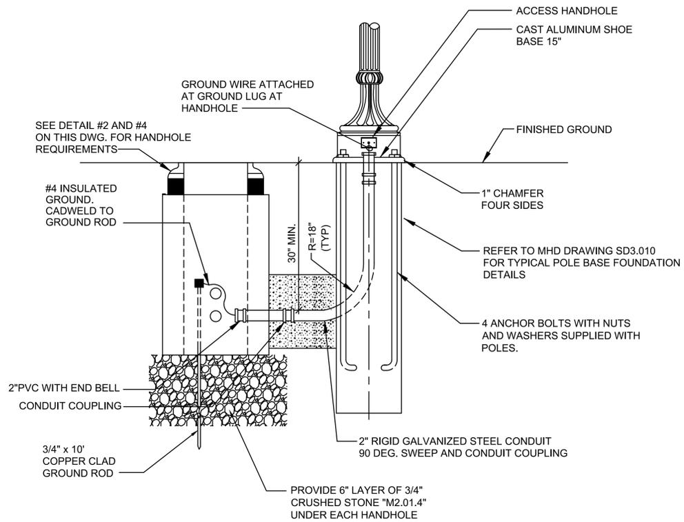
TYPICAL HANDHOLE AND POLE FOUNDATION NOT TO SCALE
