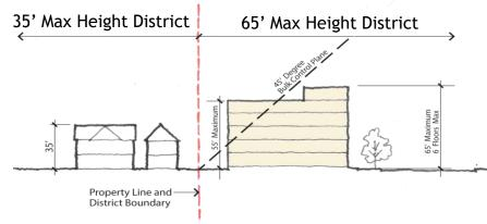
The principal cornice line facing the lower height district must be no taller than 20' above the max height in the abutting district. Anything taller than this cornice line must be set back behind a 45-degree bulk control plane, measured from the ground at the district boundary line (Section 19.52).
