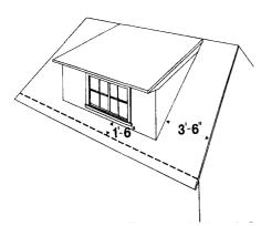
Figure 6: If the dormer meets the recommended setbacks for side (3 fl. 6 in.) and front (1 fl. 6 in.) walls, the dormer roof may start at the ridge line.
