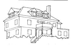
Figure 14: Matching "bookend" gable dormers added to an existing shed-roof dormer, or included as part of a gable/shed roof addition, offer a balanced appearance while increasing living space.
