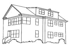
**Figure 8:** The preferred location for a larger single dormer on a gable-front building is offset toward the rear.
