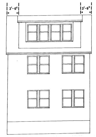
**Figure 1:** Shed-roof dormers should be setback no less than 3 ft. 6 in. from the gable end walls and 1 ft. 6 in. from the main walls underneath the eaves.
