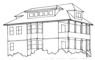
Properly designed dormers can increase the living space of an attic story while preserving the character of a building. Dormers come in a variety of styles depending upon the shape of the main roof. This duplex house with a large hipped roof has successfully increased its third-floor living space by adding three appropriately scaled hipped dormers to the side and ends of the roof.
