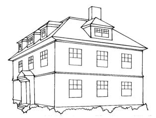
Figure 13: Gable dormers added in combinations, such as triplets, should be arranged symmetrically within the main roof so they are centered and spaced proportionally. The distance between each should be no less than one half (1/2) the width of the largest dormer.
