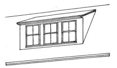
Figure 10: In general, window area, including the framework, should account for at least 50 percent of the dormer's front wall face.
