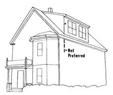
Figure 2: Setting the front wall of a dormer flush with the main wall underneath is not recommended. See Fig. 6 for the preferred 1 fl. 6 in. setback.
