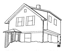
Figure 3: The front wall of a dormer should not extend beyond the main wall of the building.
