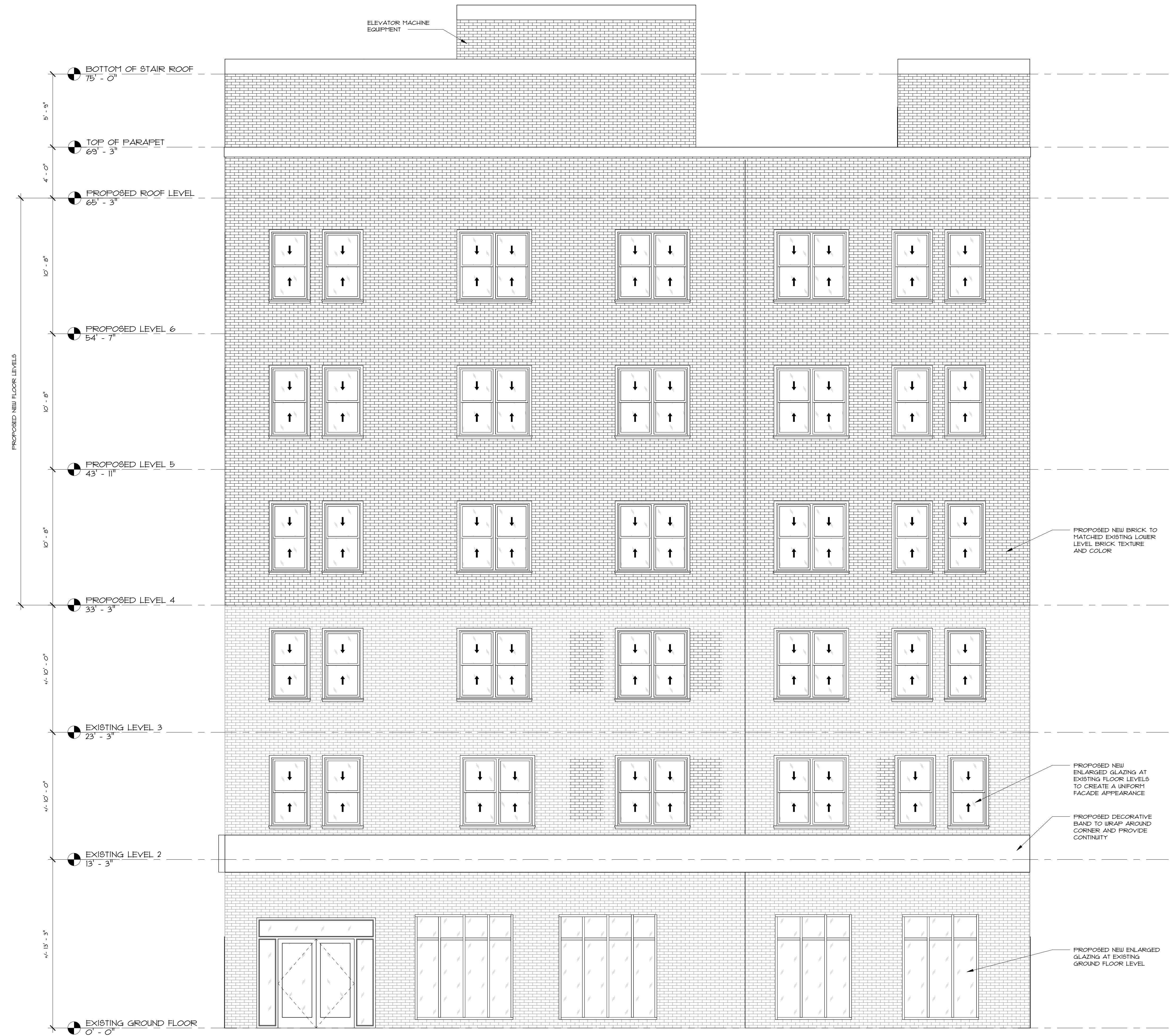
1 SD3.1 PROPOSED SOUTH EXTERIOR ELEVATION - CAMBRIDGE STREET 1/4" = 1'-0"
