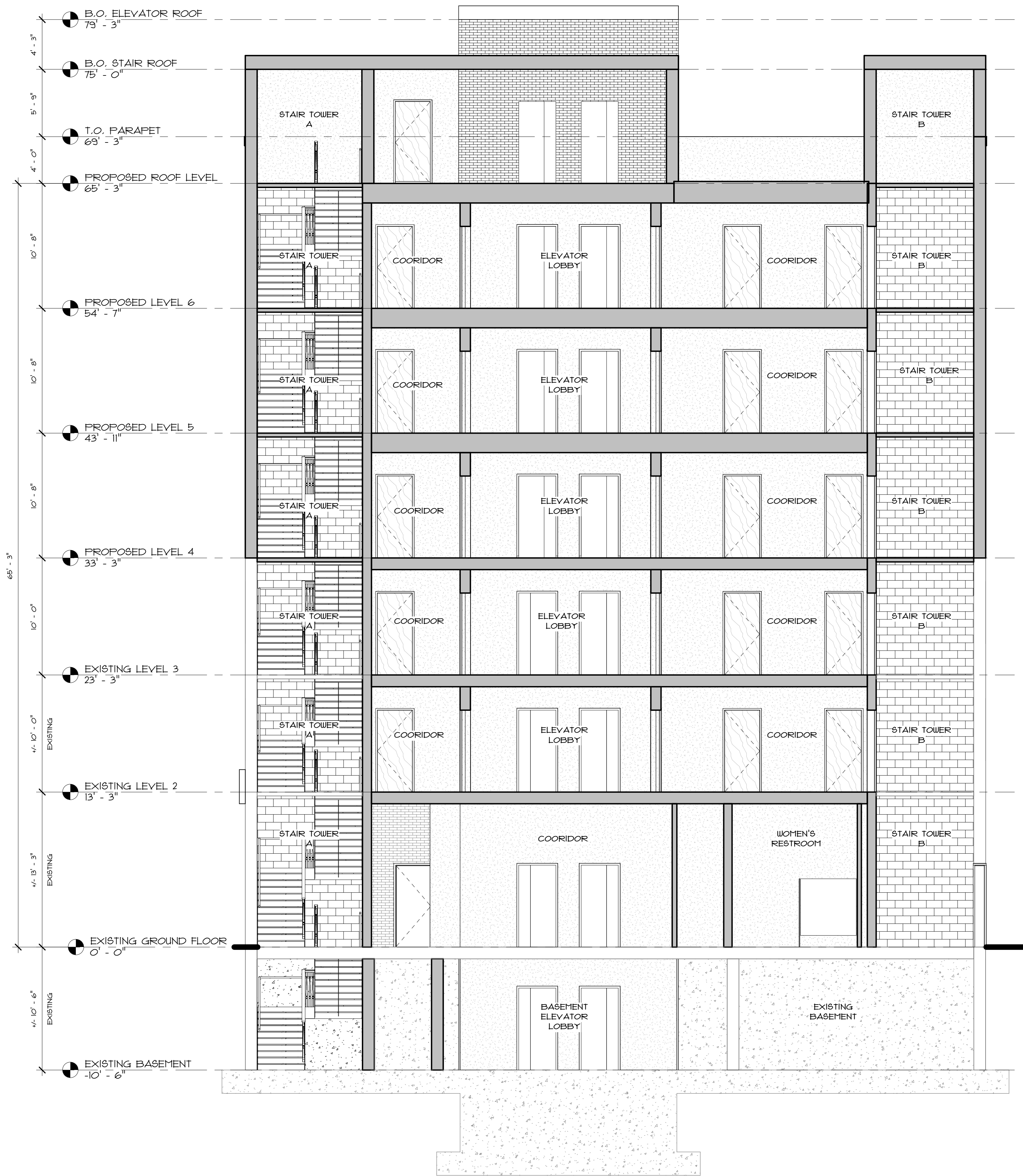
1 PRELIMINARY BUILDING LONGITUDINAL SECTION AD3.2 3/16" = 1'-0"
