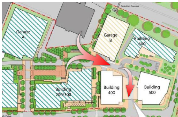
Image 6 – WNW Winds Channeled between Buildings and Deflected into the Passageway
