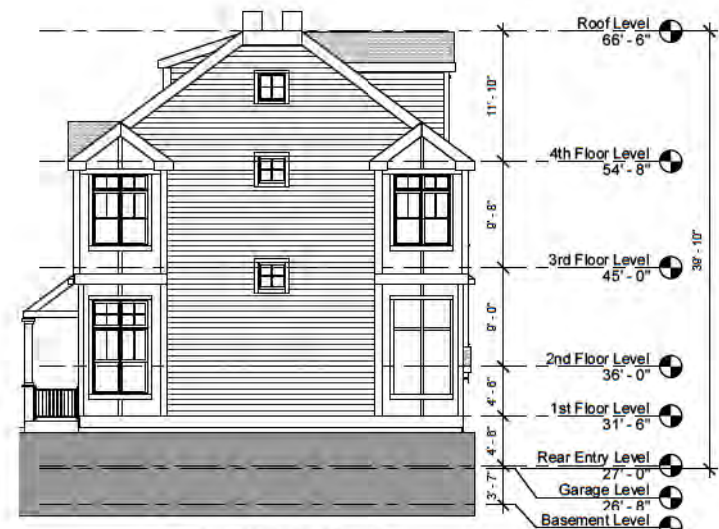
⑨ Units 28 to 29 East Elevation 1/8" = 1'-0"
