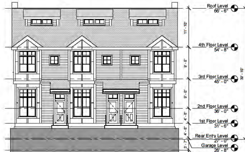
8 Units 20 to 22 South Elevation 1/8" = 1'-0"
