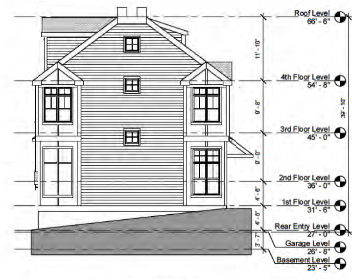
② Units 7 to 13 East Elevation 1/8" = 1'-0"
