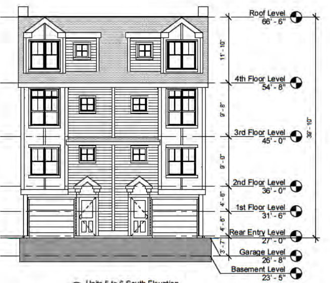
⑩ Units 5 to 6 South Elevation 1/8" = 1'-0"
