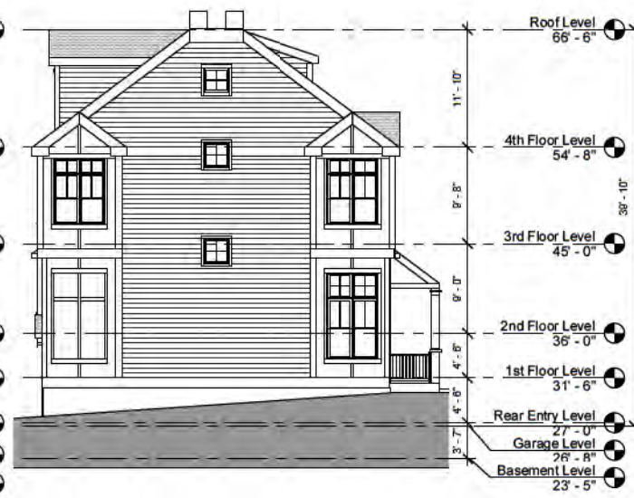
⑪ Units 23 to 25 West Elevation 1/8" = 1'-0"
