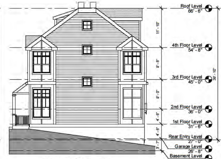
⑨ Units 26 to 27 East Elevation 1/8" = 1'-0"
