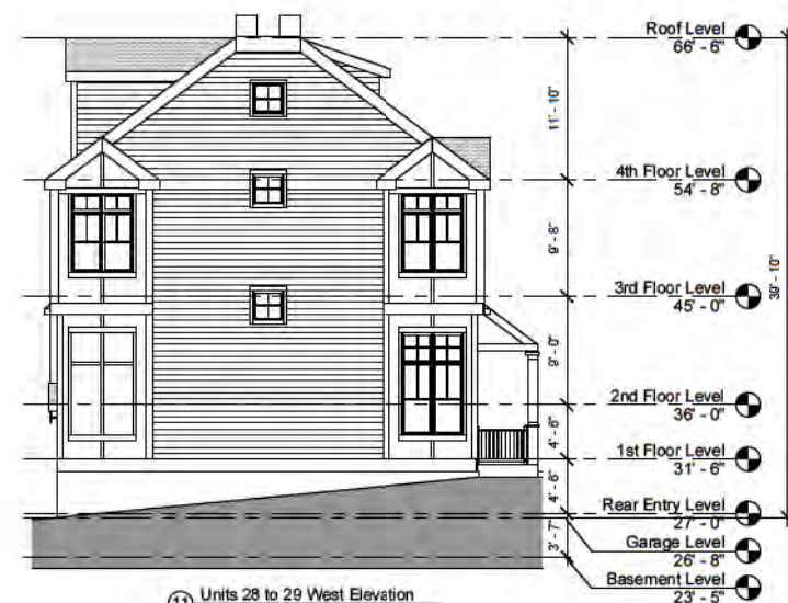
⑪ Units 28 to 29 West Elevation 1/8" = 1'-0"
