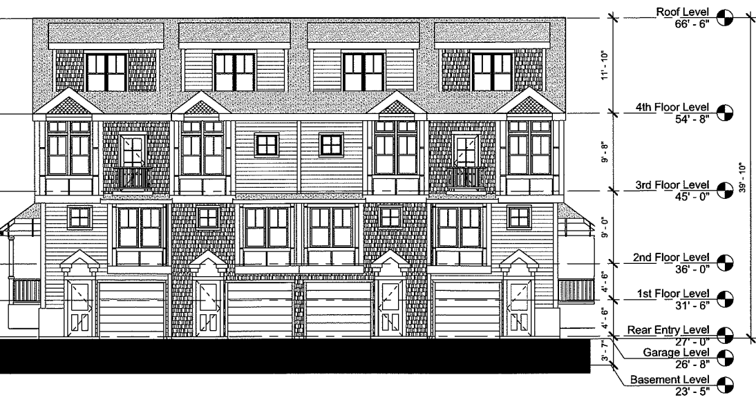
③ Units 26 to 29 North Elevation 1/8" = 1'-0"
