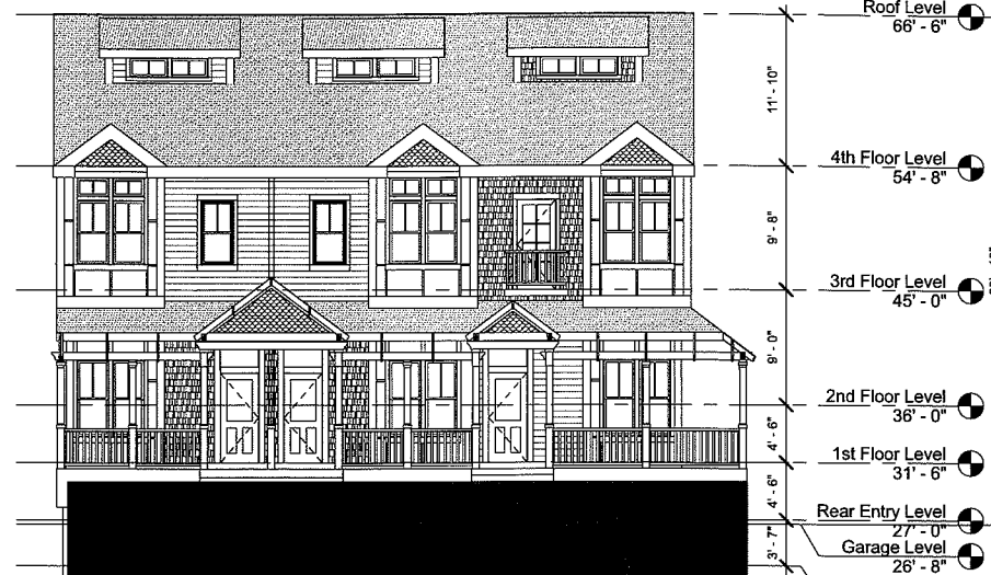
⑧ Units 23 to 25 South Elevation 1/8" = 1'-0"
