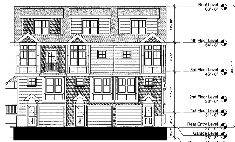
⑨ Units 23 to 25 North Elevation 1/8" = 1'-0"
