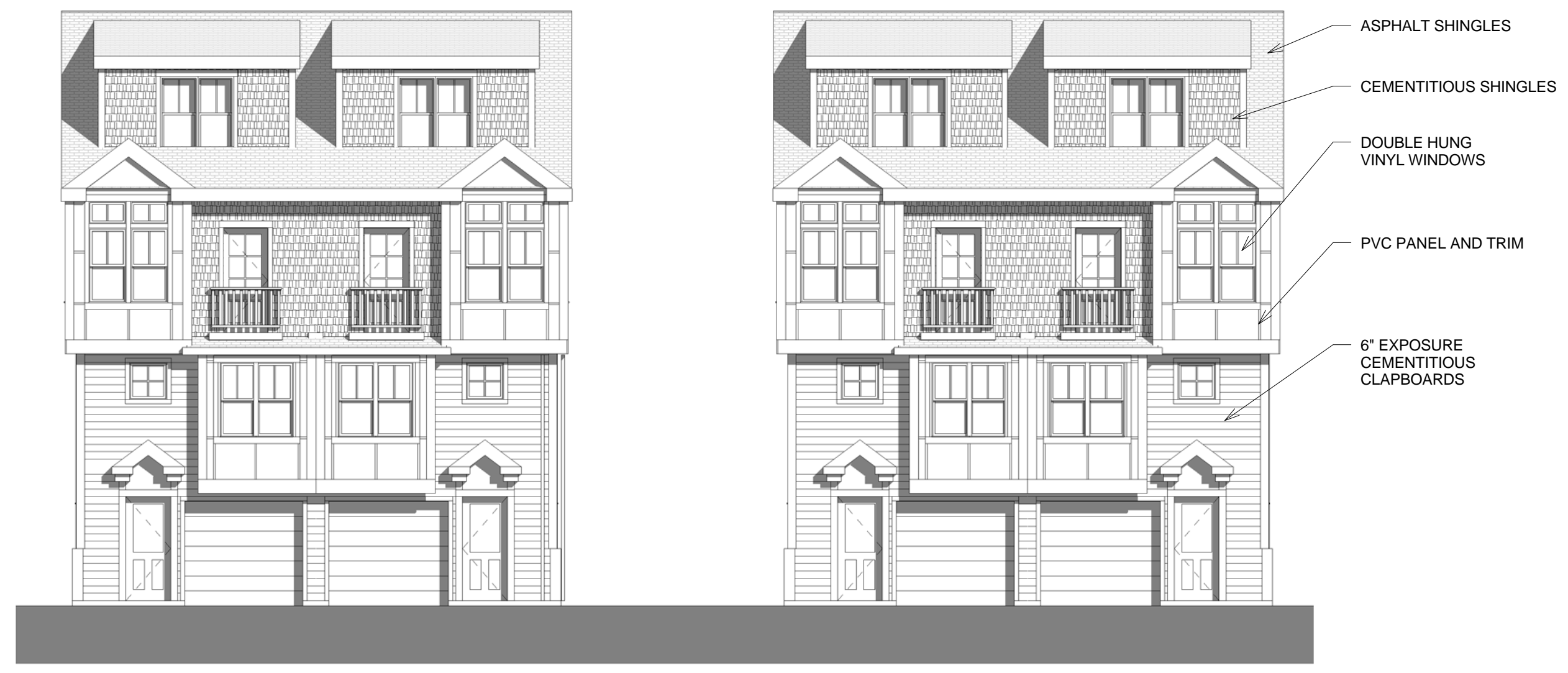
③ Units 14 to 17 South Elevation 1/8" = 1'-0"
