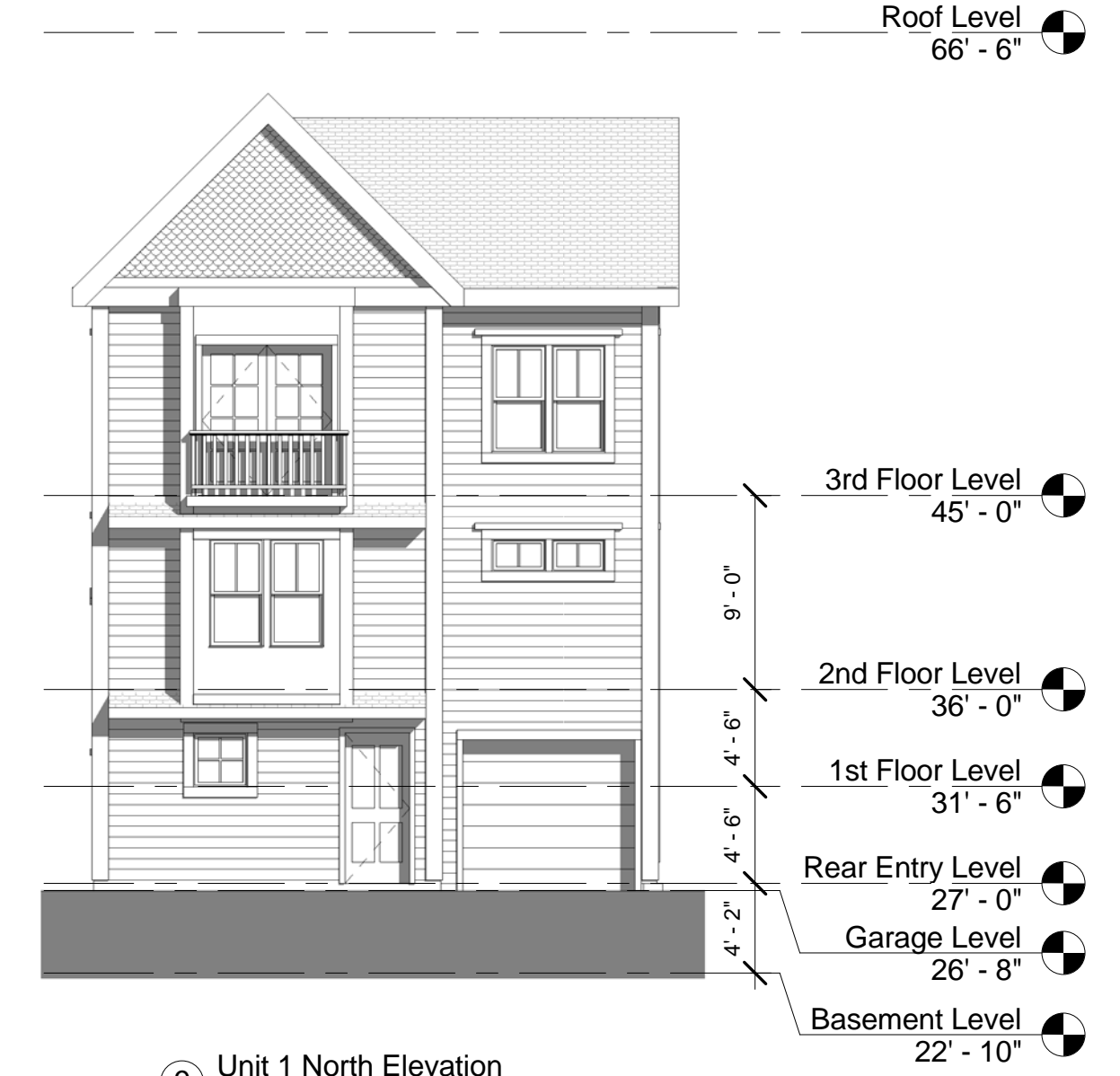
⑨ Unit 1 North Elevation 1/8" = 1'-0"
