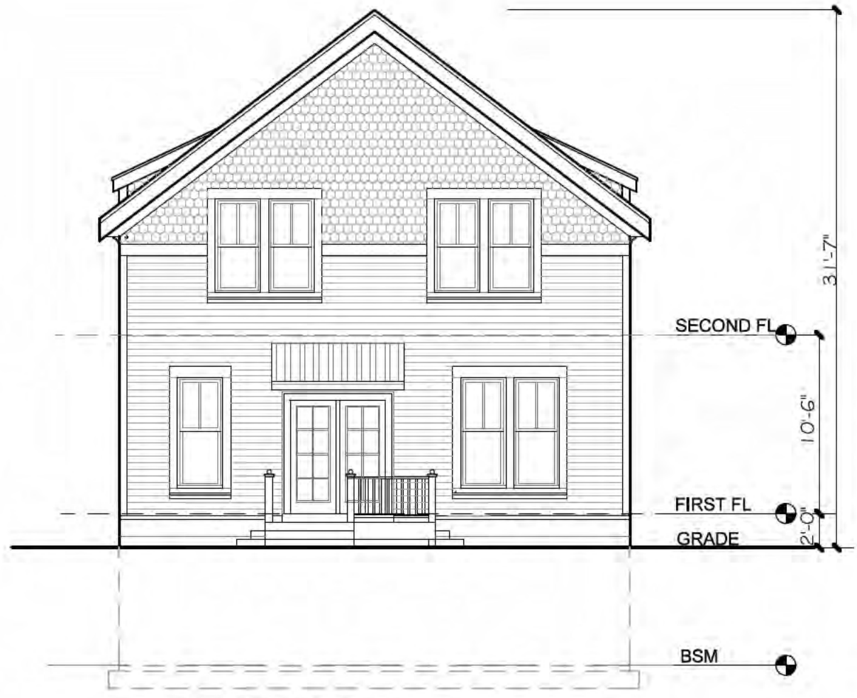
1 NEW BLDG REAR (WEST) ELEVATION SCALE: 1/8"=1'-0"
