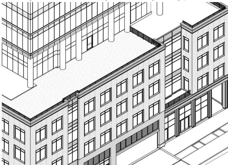
Image 5b – Removed Cornice Overhang on the Redeveloped Building (Build)
