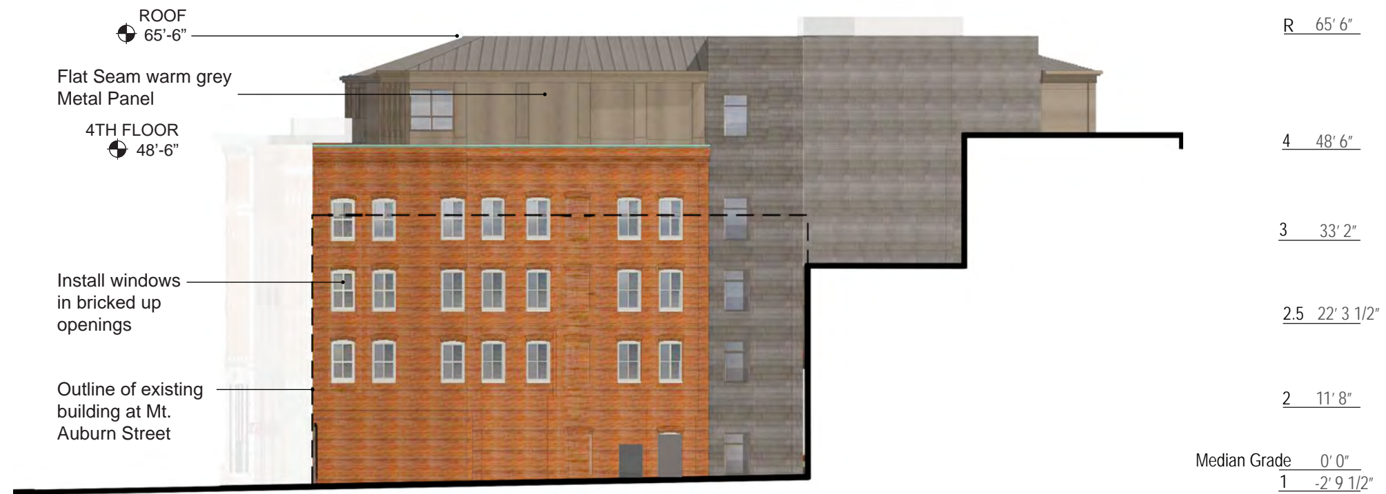
WEST ELEVATION (INTERIOR TO THE BLOCK)
