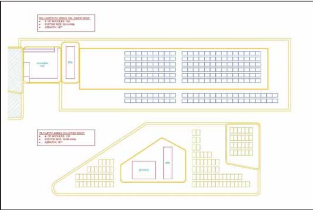
Building A – Ballasted and Tilt Up Kit Array on Lower and Upper Roofs
