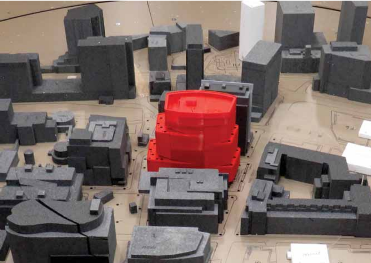
Image 2B: Wind Tunnel Study Model – Build Configuration
