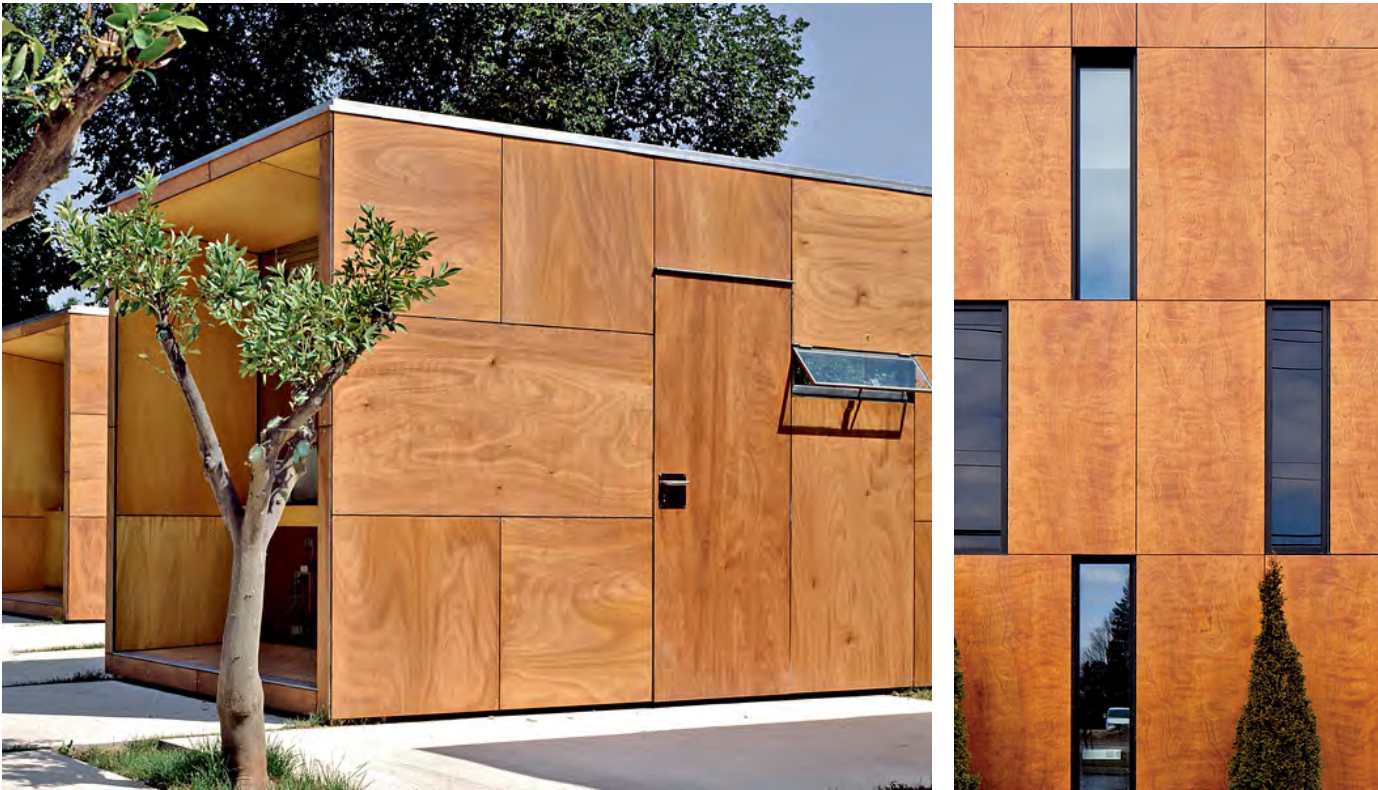
The phenolic panels contain real wood veneer, which gives inherent variation and richness to the facades. The application at New St varies from thinner slat panels to larger format panels at the New St plaza, where the full character of the graining will shine through.
