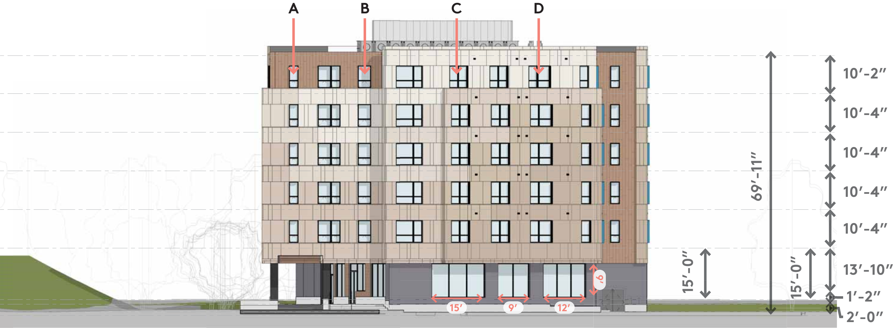
WEST ELEVATION | FACING NEW STREET
