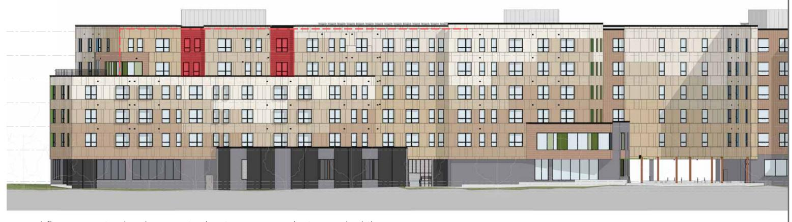
ground floor screening has been revised to incorporate glazing at the bike room, and a series of landscape screens to break up the long ground floor elevation and further integrate the project with the landscape
