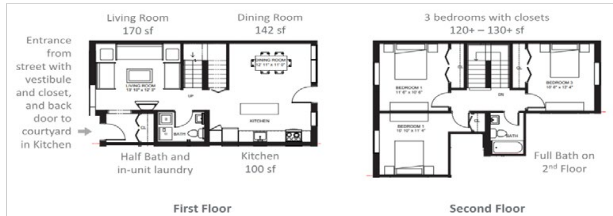
Figure 3: Typical 3-bedroom apartment layout (town-house style)
