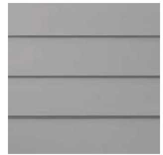
fiber cement lap siding
