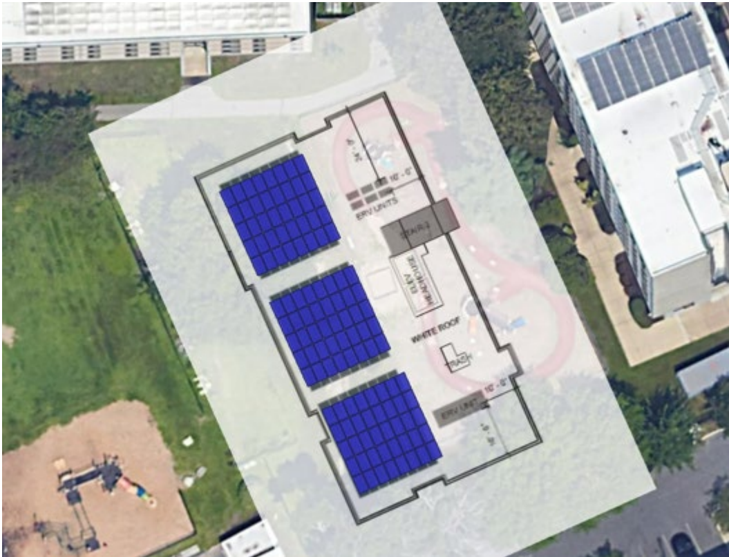
Figure 1 shows the detailed layout generated using the Helioscope PV system planning tool. PV arrays were designed to maximize available solar ready roof spaces.
