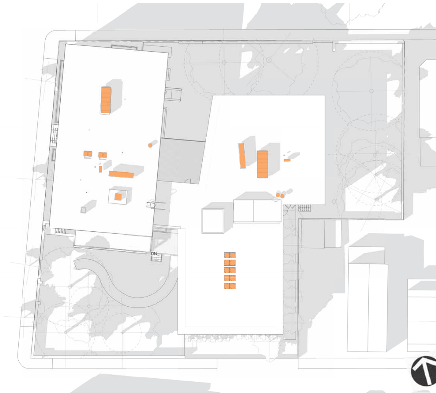
Plan View of Rooftop MEP Equipment
