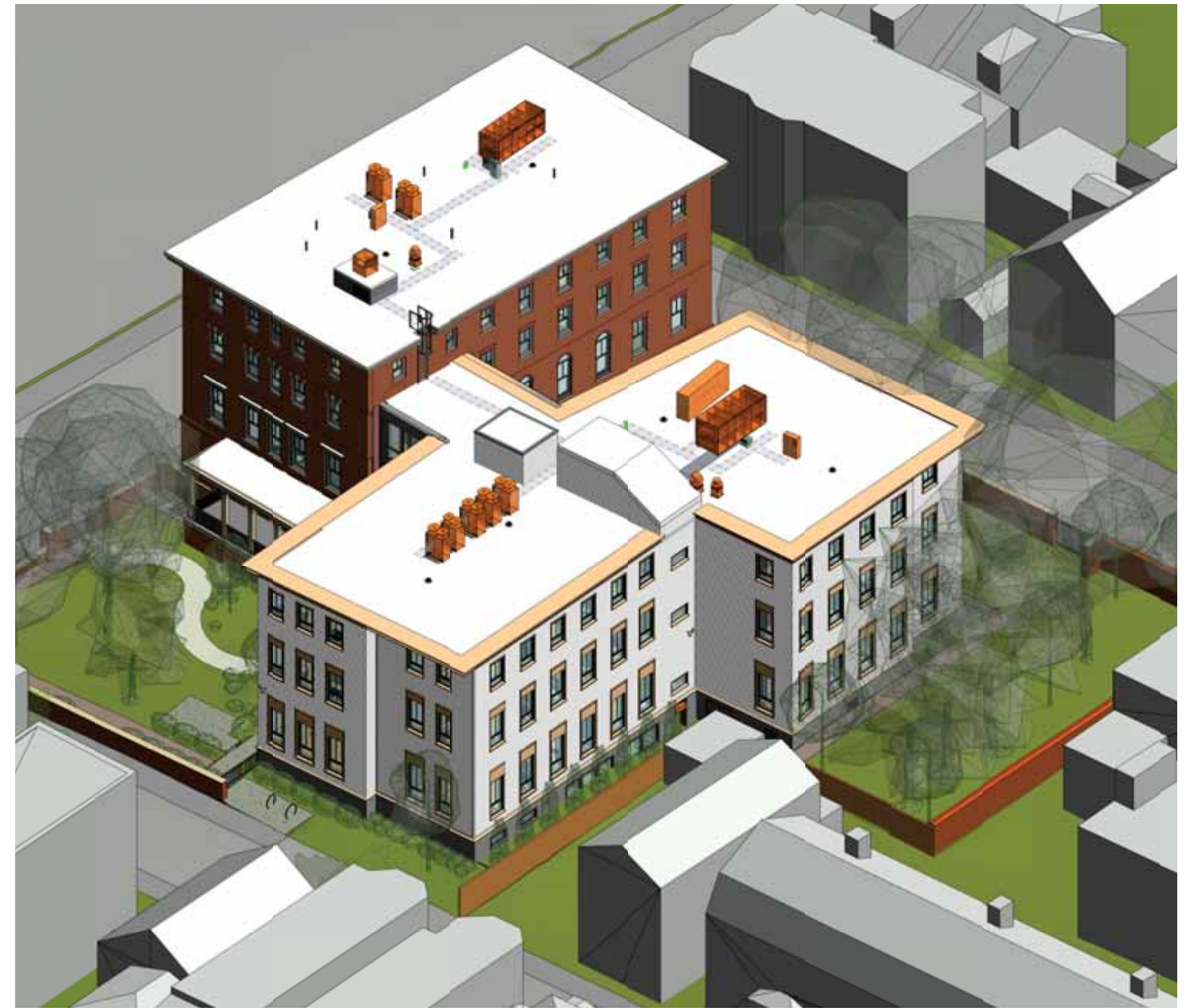
Axon View of Rooftop MEP Equipment
