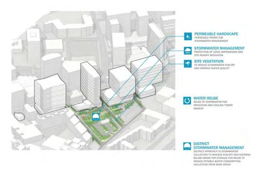
The landscape design via native vegetation and drip irrigation will achieve at least 50% reduction in potable water for irrigation. 50% of the remaining irrigation demand will be met by stormwater reuse.
