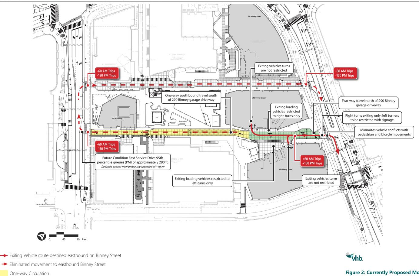
Figure 2: Currently Proposed Modified Access/Circulation Plan
