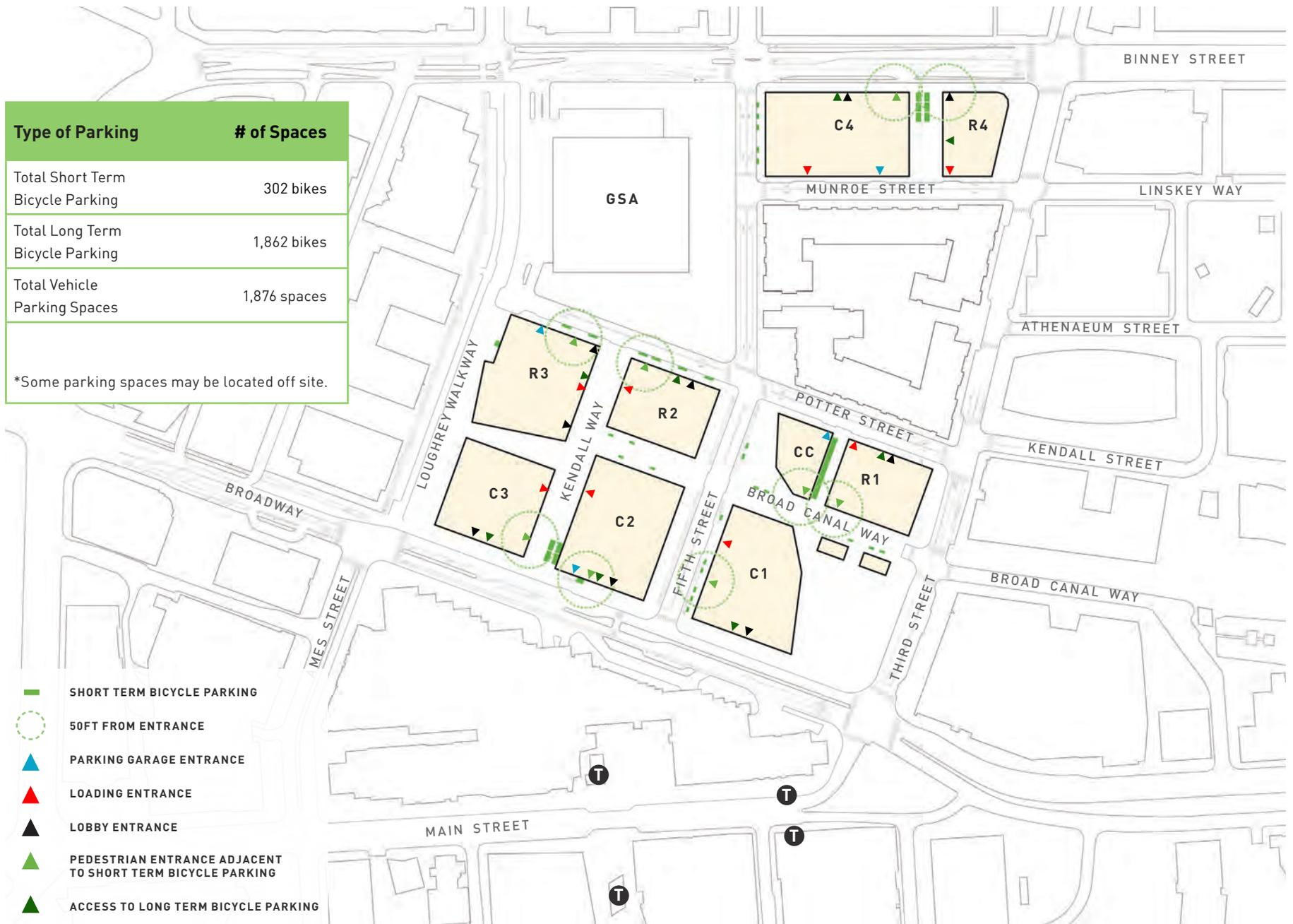
Figure C1: Vehicular and Bicycle Parking Access Plan
