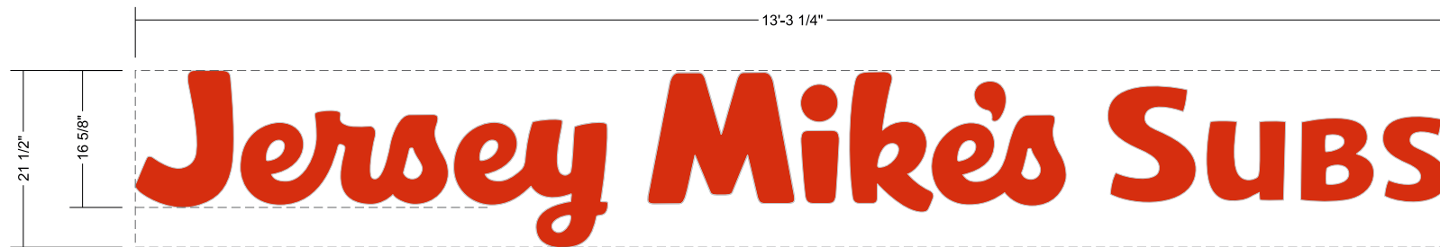
A ILLUMINATED CHANNEL LETTERS - FRONT VIEW Quantity: 1 ( 23.78 SQFT OF 24.25 SQFT PERMITTED) Scale: 1:16
