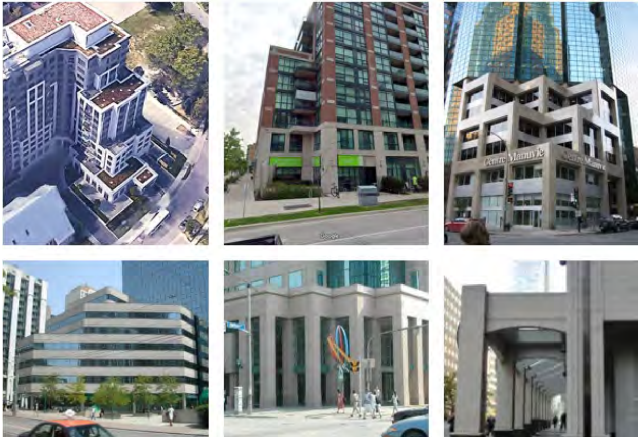
Images 6: Examples of large-scale wind control strategies - Stepped massing, Arcades/Colonnades
