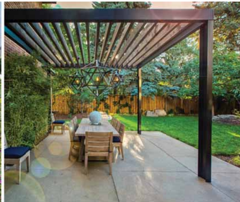
STEEL FRAMED PERGOLA W/ WOOD SLAT LOUVERS
